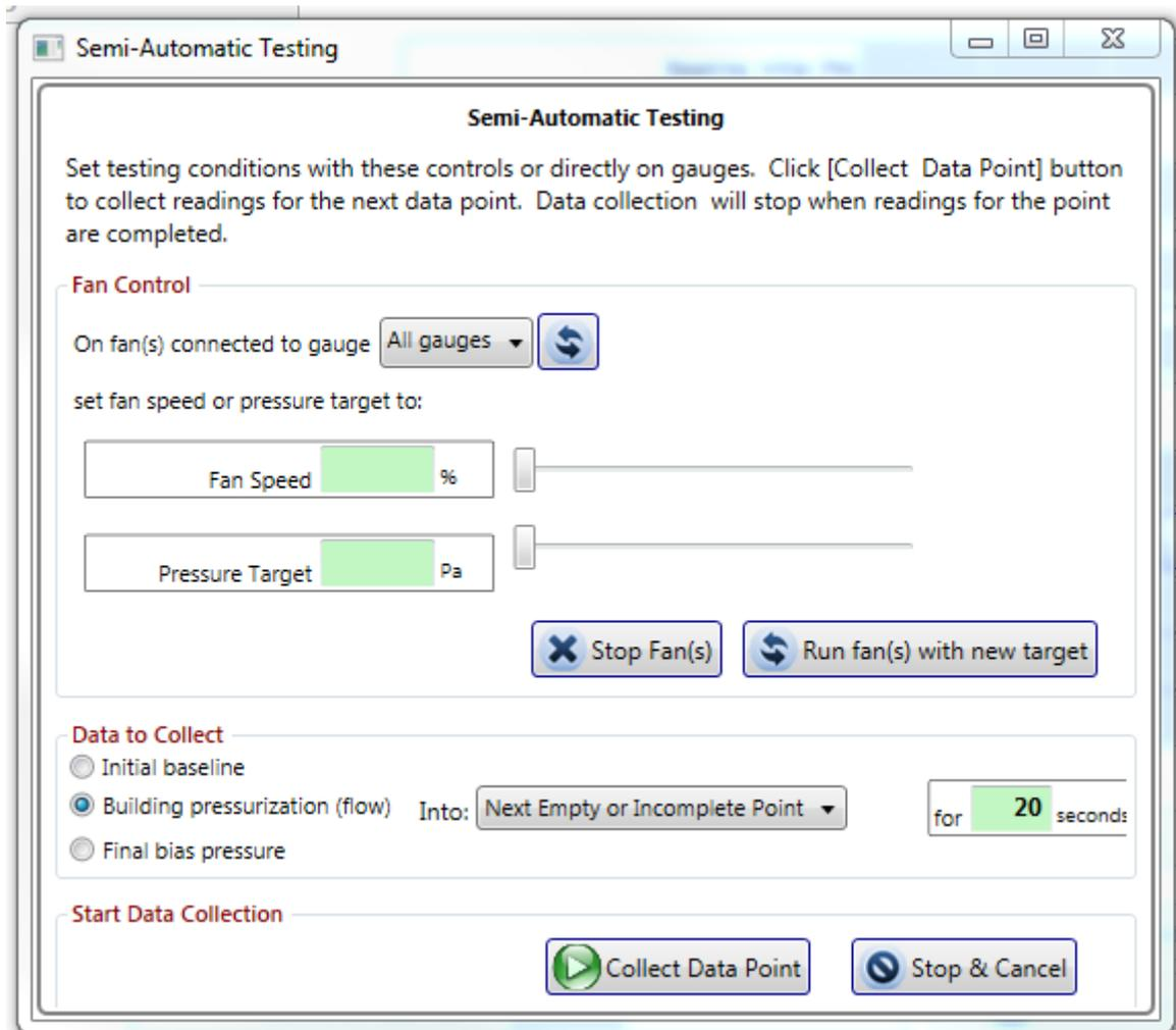
Choose which gauge you want to control (or all at the same time) and set the fan speed to a value. Click on “Run fan(s) with new target”. When the room pressure and flowrate are stable, click on “Collect Data Point”. You can choose which target point to save the data into, and you can choose how long to capture data for on each target point.
